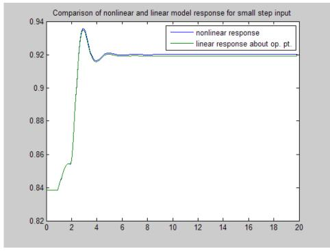
The linearized model response tracks the nonlinear model output.
